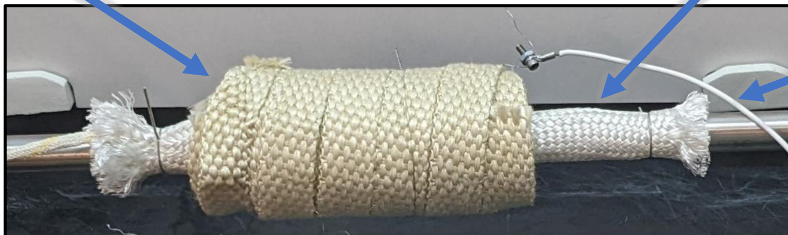
Silica Sleeve Resistant to 1260 °C
